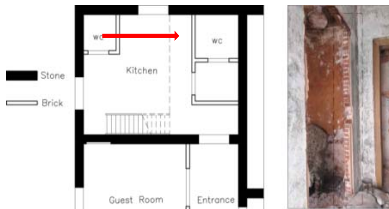
Fig. 8 Showing the materials used in the kitchen in Kaaki house abiding article 41 in the code (Hammoud J. 2016).
