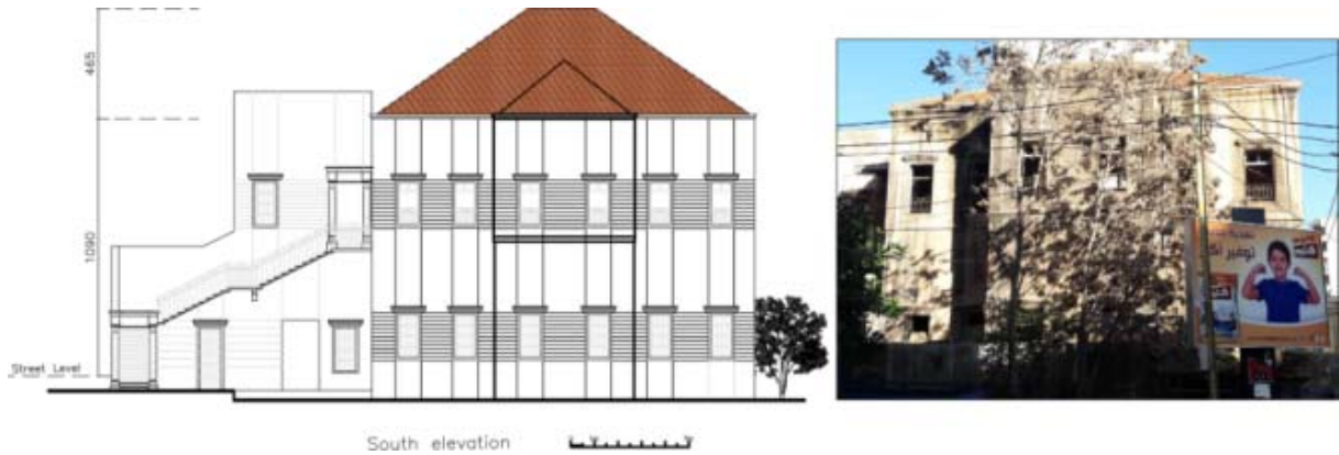
Fig. 6 The height of the Kaaki house abide with the building height code but the height of the hipped roof exceed the required height (6 cubits = 2.75meters) (AbiRached E. 2016).
