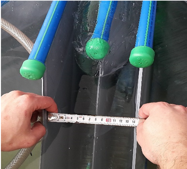
Fig. 8 Thickness of the ice walls of 14 cm from ice surface to ice surface with plate in the middle after one icing circuit with the star-shaped heat exchanger with 12 plates.
