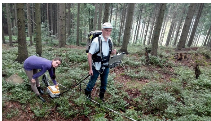
Fig. 8 Ground penetrating radar (RAMAC/GPR) with an 800 MHz antenna (GPR field measurement method).
