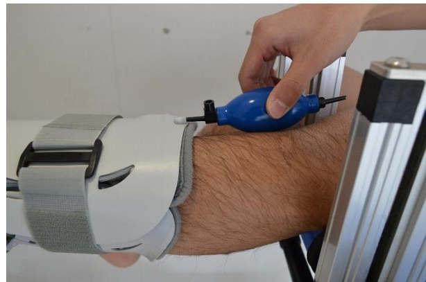
Fig. 5 Inflating air into airbag with hand-pump.
