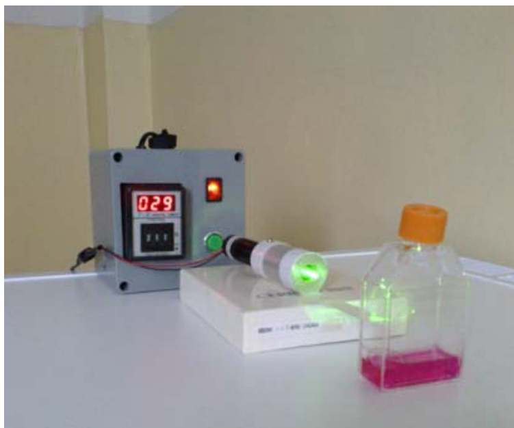
Fig. 1 A device for radiation protection of biological objects with the use of a laser module with the wave length of 532 nm.
