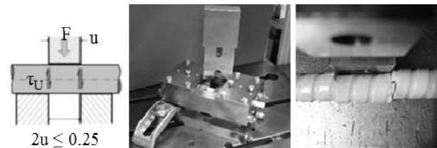
Fig. 7 Determination of shear strength according to ACI Method B4 (left: scheme; middle: device; right: specimen after testing).
