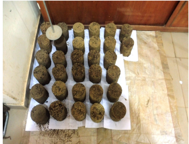
Fig. 3 Compacted specimens for UCS test.
