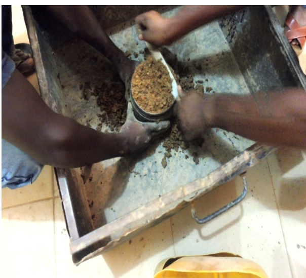
Fig. 2 Soil in mould for compaction and CBR tests.
