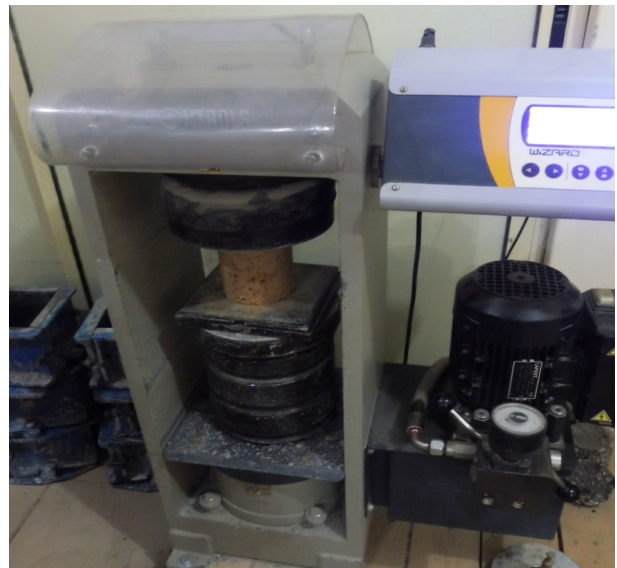
Fig. 4 Specimen for UCS in compression machine.
