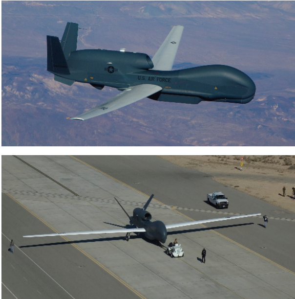
Fig. 3 Global Hawk RQ-4; top: RQ-4 flying; bottom: RQ-4 size (40 m RQ-4B wingspan, 35 m RQ-4A wingspan) [10, 11].
