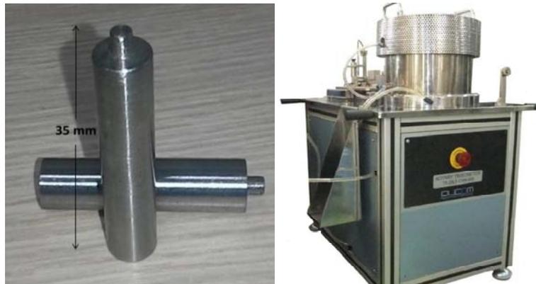
**Fig. 1** Test specimen used in wear testing and pin on disk tribometer.
