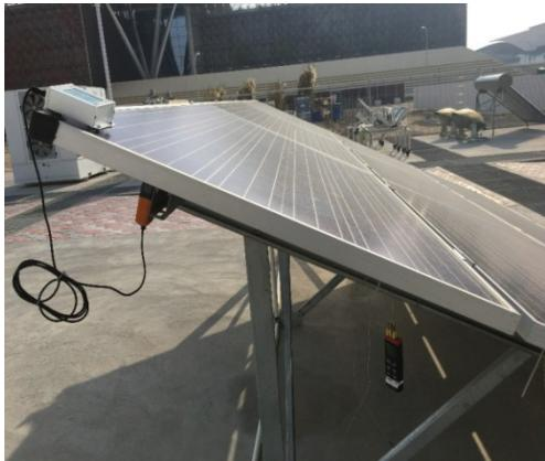
**Fig. 5** Photographic view of outdoor setup for testing polycrystalline PV module at GORD's Technohub.
