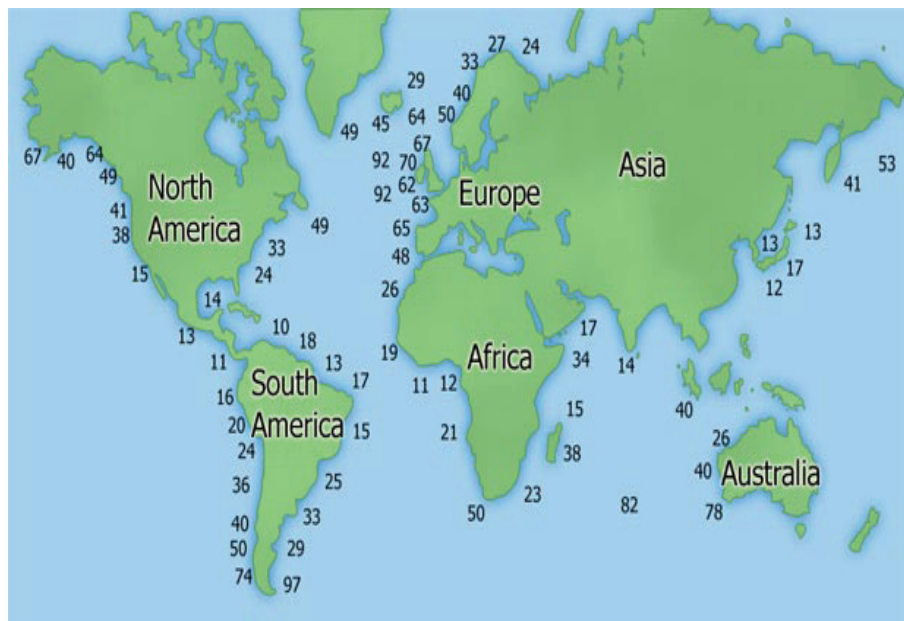
Fig. 2 Wave power distributions in the world with the unit kW/m (US Dept. of ENERGY).
