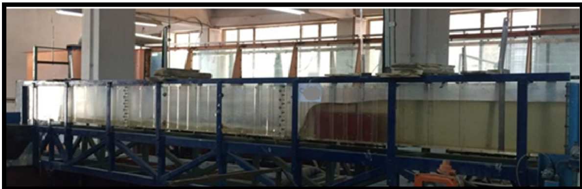
Fig. 2 Photograph showing the laboratory flume with broad crested weir.
