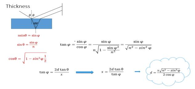
Above theory is related to thickness of glass found by snels and lambert law and the new theory which make from are manipulation on trigonometric [6]. The main variation are the main reflections angels  $\theta$  and  $\phi$ , then you earn thickness (d) with relation to them.
