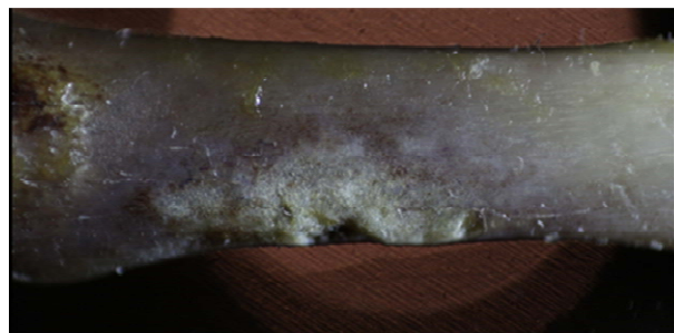
Fig. 1 Bone with presence of compound PMMA/ZINC/ \text{CaCO}_3 .
