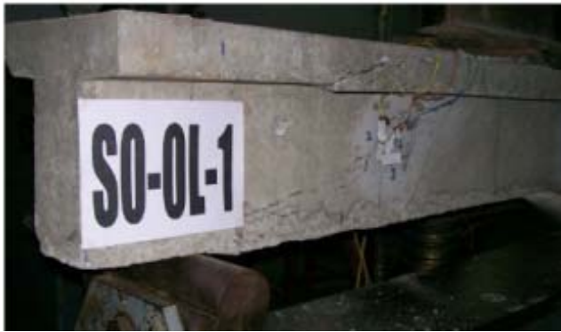
(a) Shear failure
