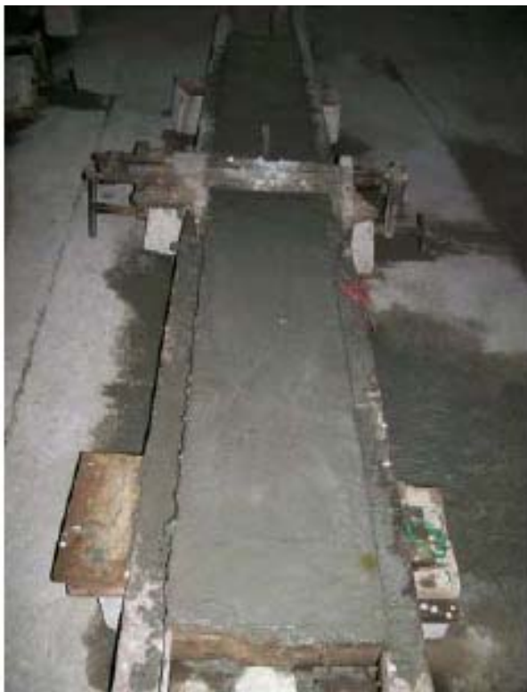
(c) Beam specimen after casting.
