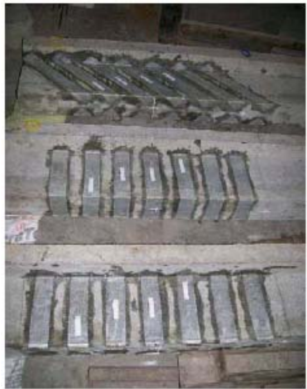
(d) Strengthened specimen with GFRP strips.
