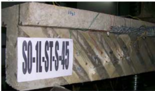
(c) Debonding and rupture failure of GFRP strips
