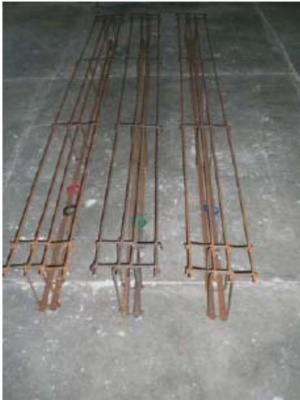
(a) Cages with strain gauges in longitudinal steel.
