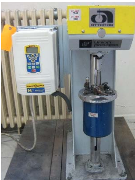
Fig. 3 Attritor mill used for mechanical grinding.
