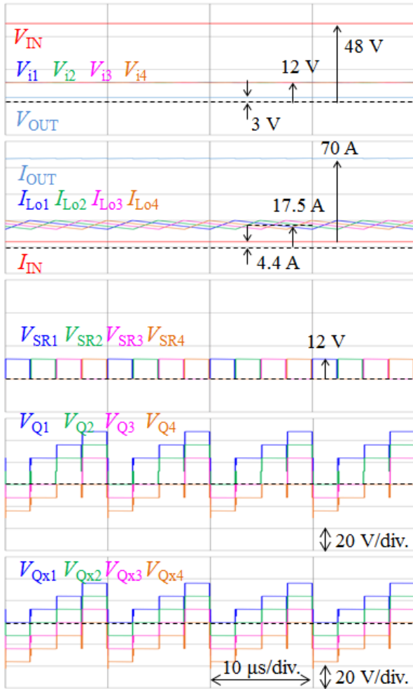
Fig. 10 Simulation result for 48 V-3 V non-isolated multicellular converter using four cell converters.
