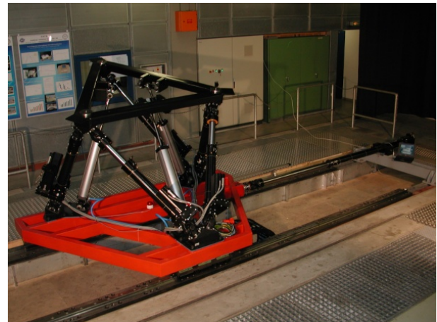
Fig. 9 Expansion of the hexapod-system of the IFAS-simulator.
