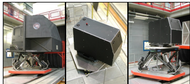
Fig. 19 Driving simulators in 7-, 1- and 8-DOF configuration.
