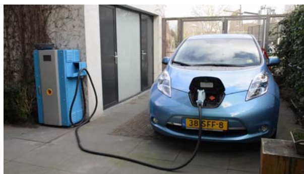
Fig. 5 DC V2G charge with a Nissan LEAF.
