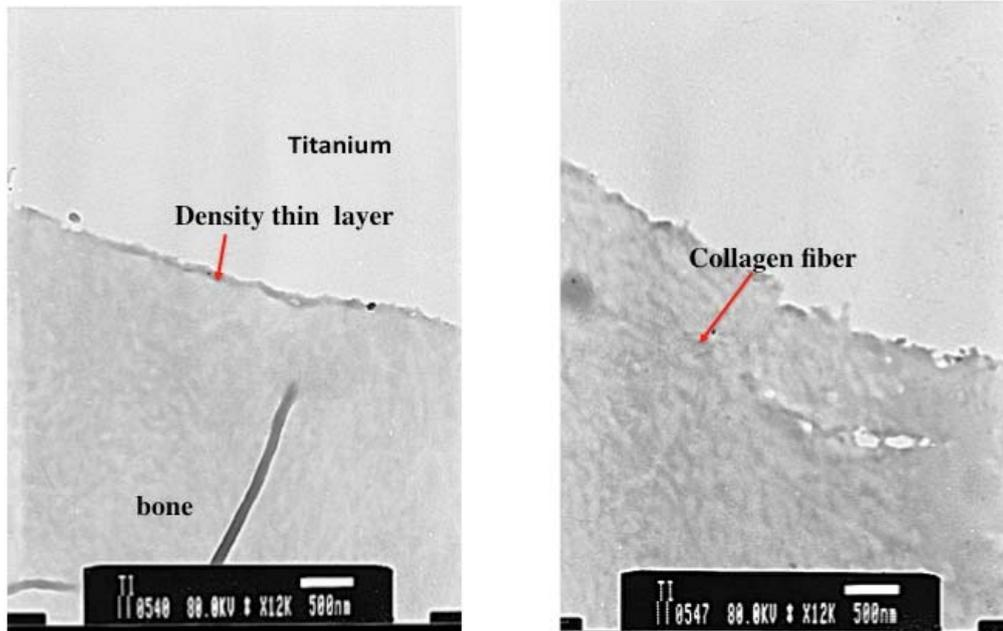
Fig. 4 TEM showed an extremely thin-density layer responding to the titanium at the surface of the bone.
