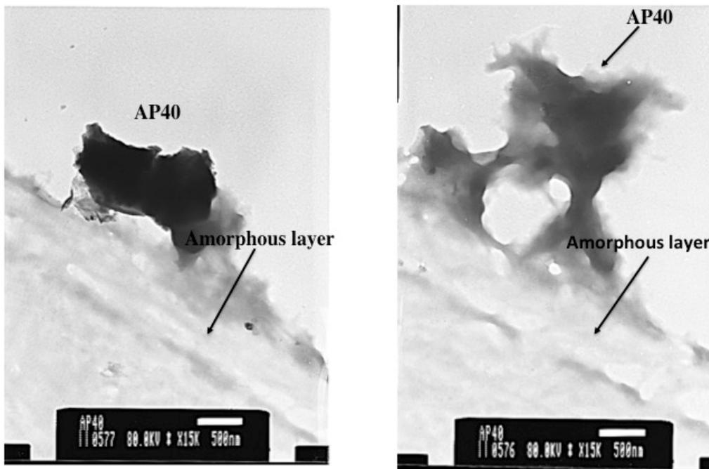
Fig. 8 TEM showed that AP40 bonded directly to the bone; however, we observed an amorphous layer between AP40 and the bone.
