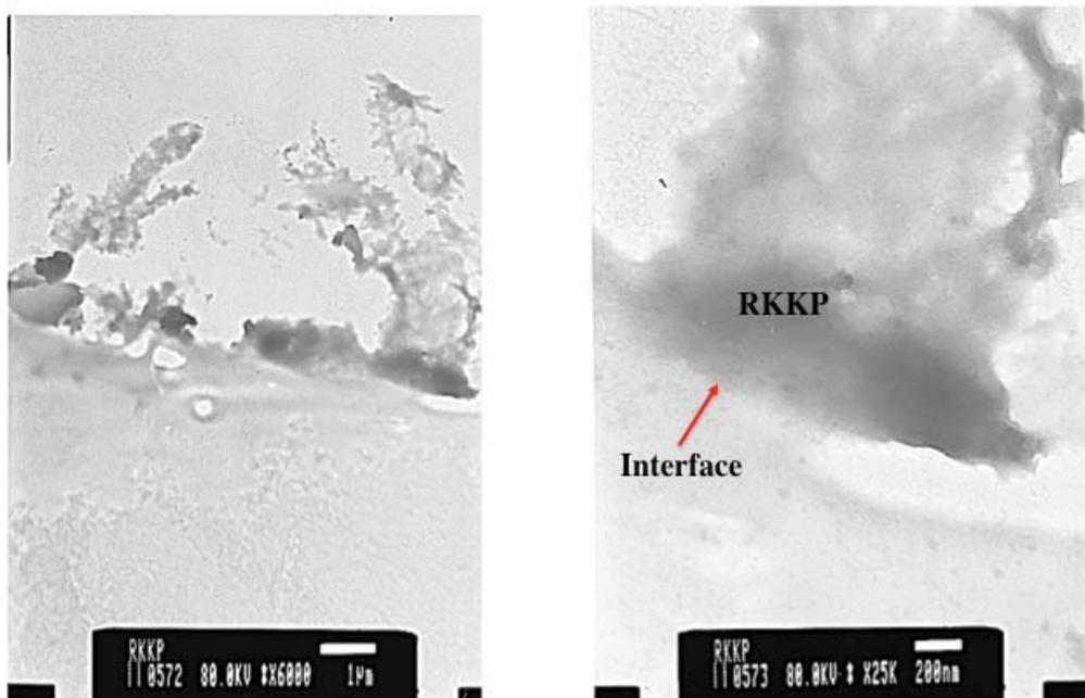
**Fig. 10** TEM showed that RKKP extends to the bone at the interface (directly bound to the bone).
