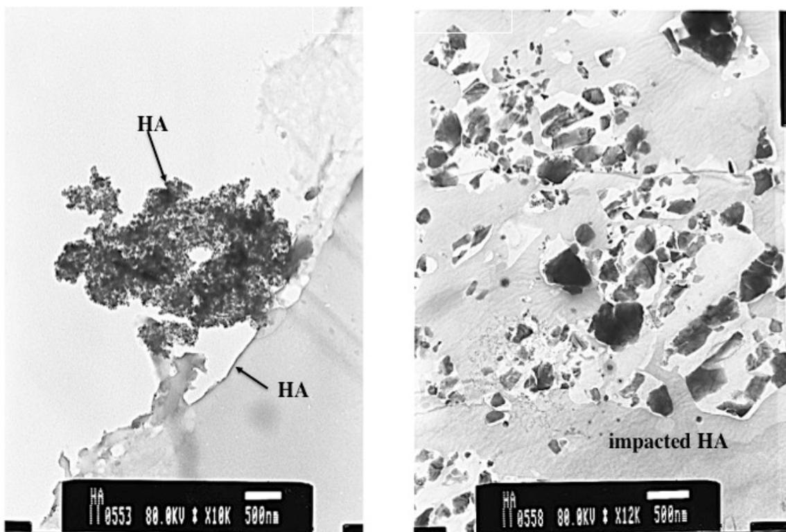
**Fig. 6** TEM showed that HA bonded directly to the bone; however, it became partially separated, and some HA particles remaining in the bone can be seen.
