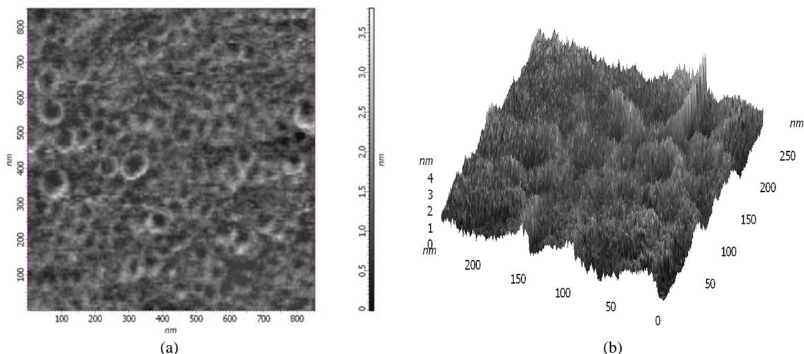
**Fig. 2** The AFM two-(a) and three-dimensional (b) image of nanoparticles based on  $\text{Fe}^{\text{III}}_x(\text{acac})_y18\text{C}6_m(\text{H}_2\text{O})_n$  formed on the surface of modified silicone.
