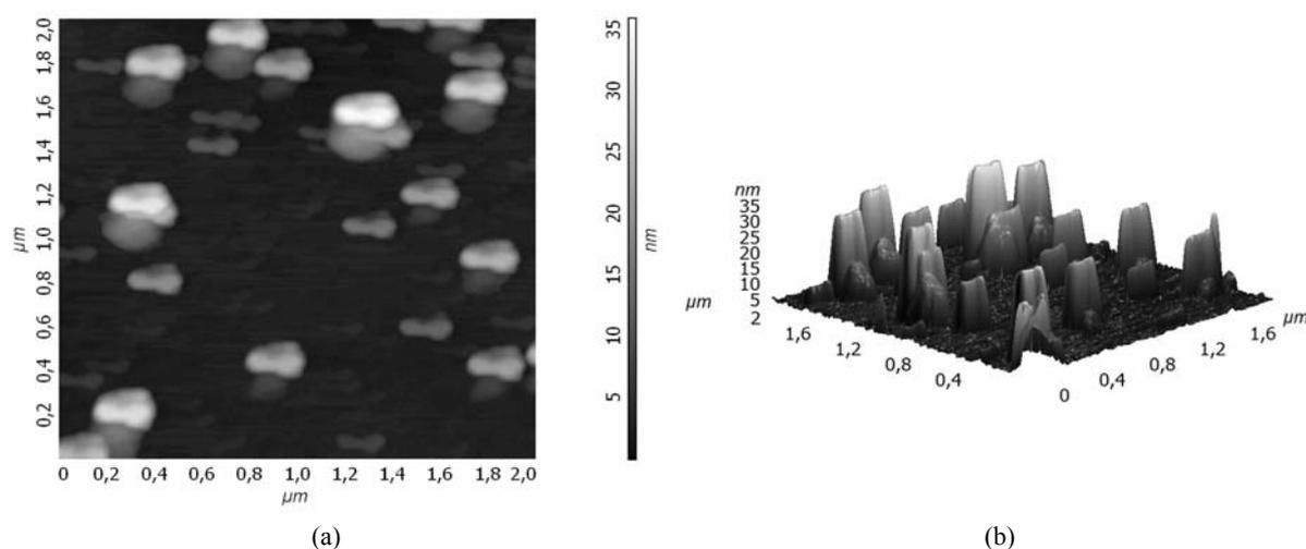
Fig. 4 The AFM two- (a) and three-dimensional (b) image of nanoparticles based on  $\text{Ni}_2(\text{AcO})_3(\text{acac})\cdot\text{NMP}\cdot 2\text{H}_2\text{O}$  formed on the hydrophobic surface of modified silicone.
