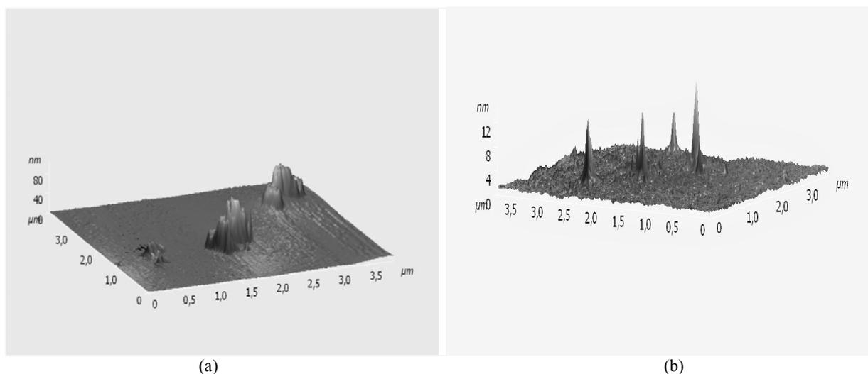
**Fig. 6** a—the AFM three-dimensional image ( $5.0 \times 5.0(\mu m)$ ) of the structures ( $h \sim 80-100$  nm) formed on a surface of modified silicone based on triple complexes  $Ni(acac)_2 \cdot NMP \cdot PhOH$ , b—AFM three-dimensional image ( $3.5 \times 3.5(\mu m)$ ) of the structures ( $h \sim 12$  nm) formed on a surface of modified silicone based on binary complexes  $\{Ni(acac)_2 \cdot NMP\}$ .
