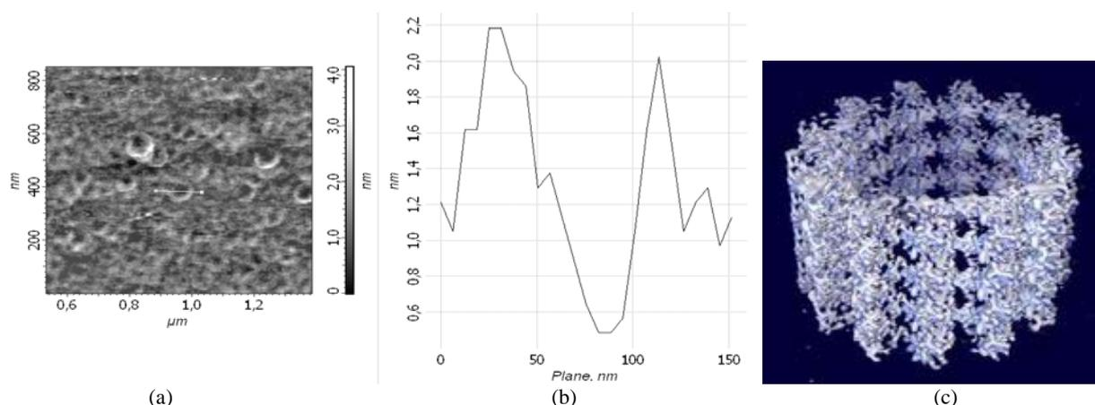
**Fig. 3** The AFM two-dimensional image (a) of nanoparticles based on  $\text{Fe}^{\text{III}}_x(\text{acac})_y18\text{C}6_m(\text{H}_2\text{O})_n$  formed on the hydrophobic surface of modified silicone. The section of a circular shape with fixed length and orientation is about 50-80 nm (b). The structure of the cell microtubules (c).
