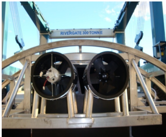
Fig. 4 Two generators, one in each air duct.
