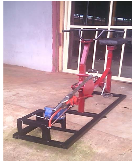
Fig. 2 Improved Pedal Powered Hacksaw Machine Developed.
