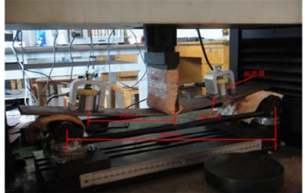
Fig. 3 Three point bending test.
