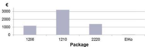
Fig. 17 Cost comparison of different DC link capacitor solutions (MLCC vs. electrolytic capacitors).
