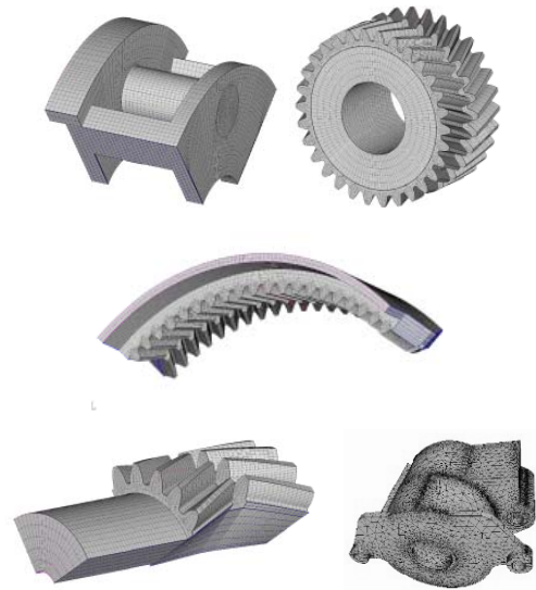
Fig. 17 FE-models for integrated stiffness calculation and analyze, bottom: external FE-model of housing calculation.
