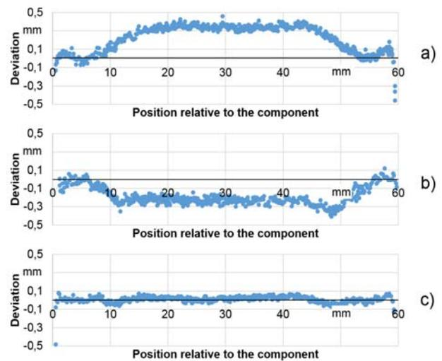
**Fig. 4** Measurement data of the thin strut of the frame with (a) no compensation, (b) a pre-deformation of 0.4 mm and (c) a pre-deformation of 0.2 mm.
