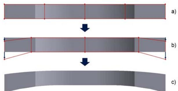
**Fig. 3** Example for the application of the FFD: (a) non-deformed cuboid and part, (b) deformed cuboid and (c) deformed part.
