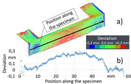
**Fig. 6** False color plot of the measurement data of the laser-scan of an uncompensated specimen (a) and evaluation of the deformation along the specimen (b).
