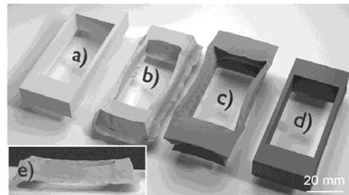
**Fig. 5** Pre-deformation procedure by inversion of the simulation results: (a) initial geometry, (b) result of the 1st iteration, (c) pre-deformed part (5th iteration), (d) result of the 5th iteration and (e) side view of the result of the 1st iteration with the apparent curling effect. The warpage is magnified 50 times.
