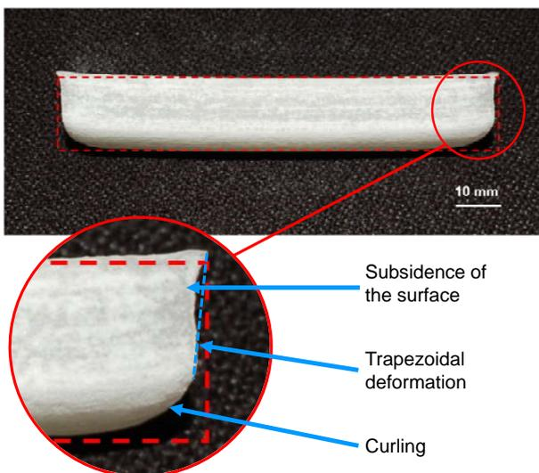
**Fig. 1** Deformation of a cuboid produced with 3DP.
