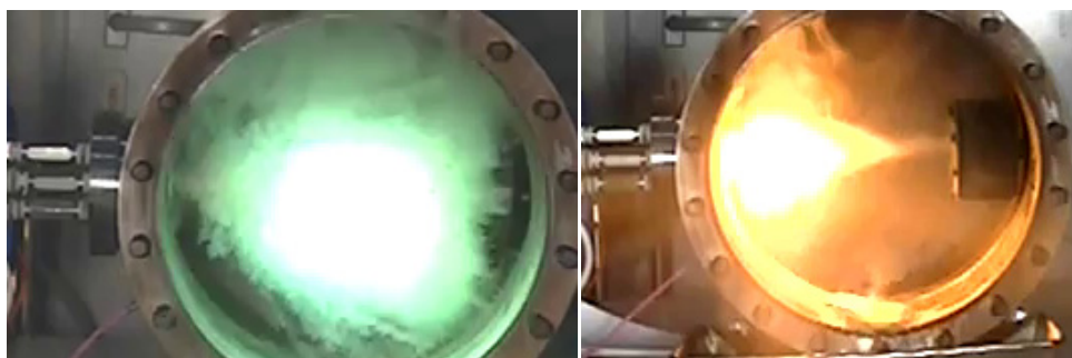
Fig. 3 The impinging tests of the hypergolic with 98%+ HTP liquid propellants; left is MEA (monoethanolamine) catalytically promoted with copper chloride and in the right picture is the mixture of MEA with dimethylamine promoted with strong reducing agent (sodium borohydride) (IoA).
