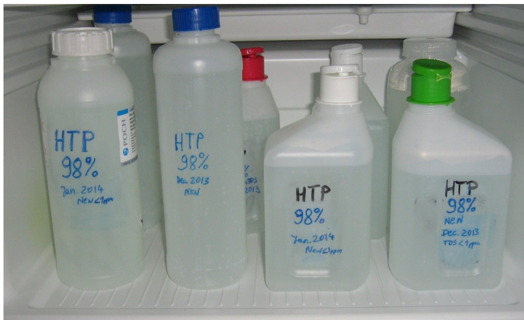
Fig. 2 The HDPE containers with one litre samples of 98%+ grade, non stabilised HTP prepared at IoA.
