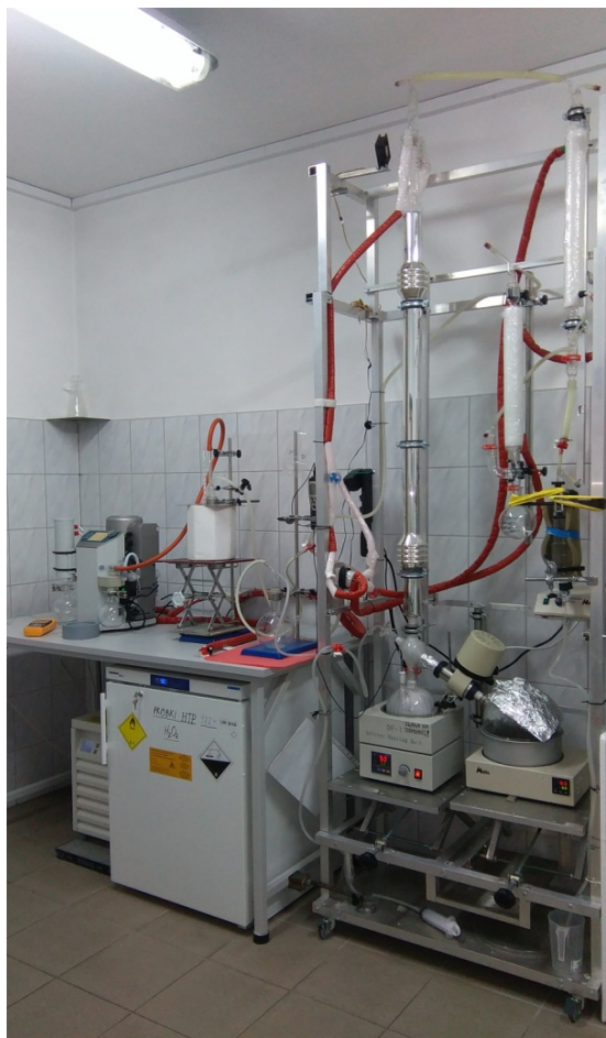
Fig. 1 The laboratory apparatus for preparing 98%+ HTP at IoA research facility.
