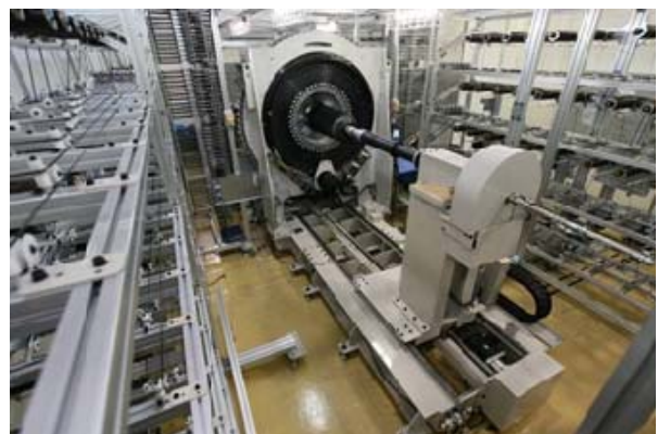
Fig. 8 Automatic MFW machine with 180 bobbins.
