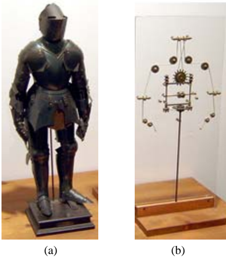
Fig. 3 Knight's robot Leonardo da Vinci: (a) moving outer armor, inside (b) the system drive [3].
