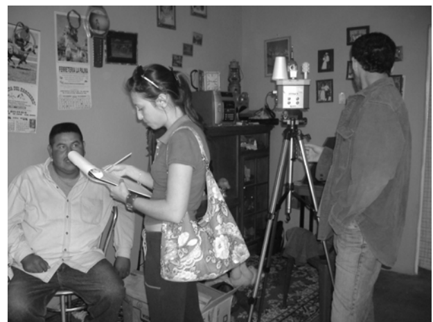
Fig. 5 Field surveys in houses. A student is applying a questionnaire while indoor thermal conditions are measured.
