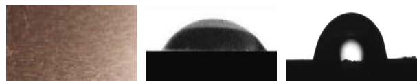
Fig. 11 Planar micro-scale profiled surface, contact angle on a plain and a micro-scale profiled plate.
